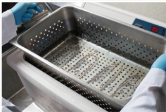
An ultrasonic, aqueous cleaning removes all soils and contaminants from wire.
