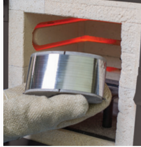
Heat-treatment sets the archform shape to wire.
